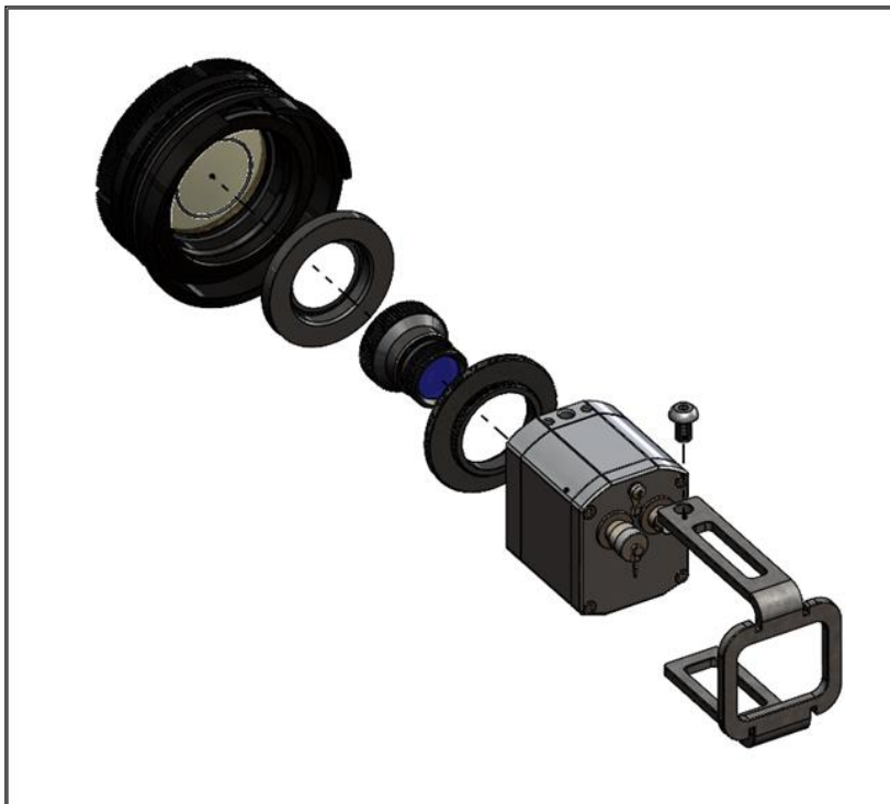
Figure 19: Assembling of the 80° optics
