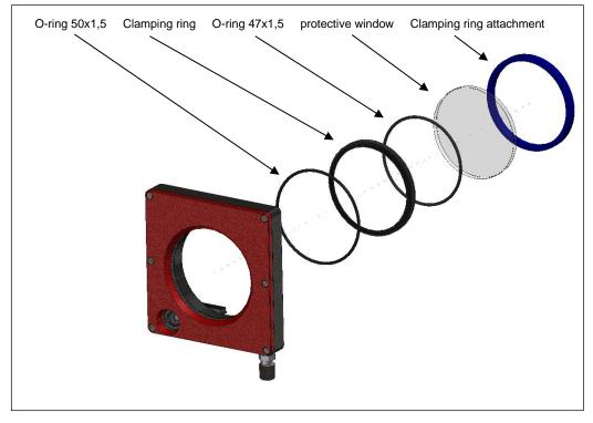
Figure 31: Assembly protective window
