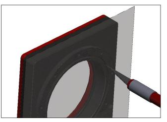
Figure 28: Cut the protective foil along the nut inner surface
