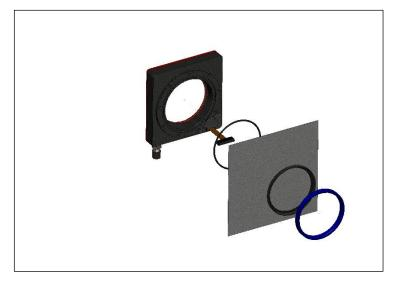
Figure 26: Insert new protective foil
