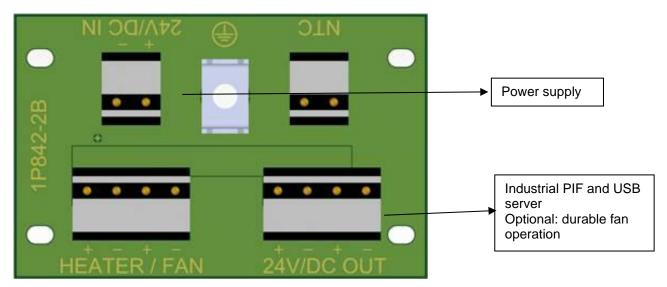
Figure 3: Connection circuit board
