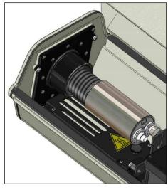
Figure 15: Xi camera mounted in adapter plate
