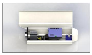
Figure 14: Fully assembled PI camera in outdoor protective housing
