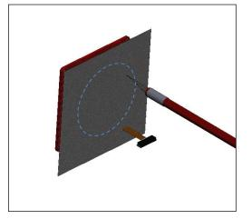
Figure 27: Cut the protective foil with the scalpel
