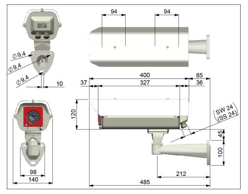
Figure 1: Dimensions [mm] with wall mount
