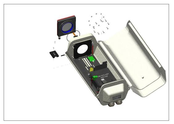
Figure 24: Remove air purge laminar
