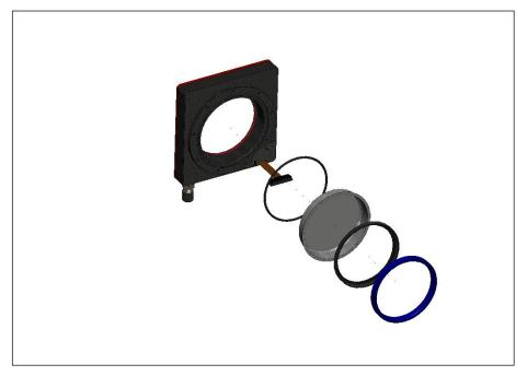
Figure 25: Remove old protective foil
