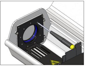
Figure 23: Loosen 9 screws from the adapter plate
