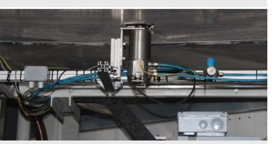
optris PI thermal imaging camera, water-cooled in industrial protective housing can be used at temperatures of up to 315 °C.
