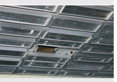
Heating field comprising radiant heaters, arranged in columns and rows. One heating field was removed for the viewing field of the camera.
