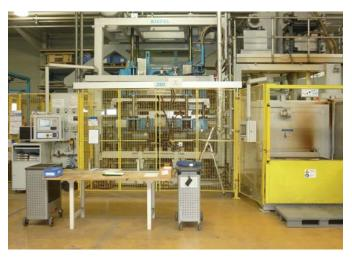
A Kiefel deep-drawing system is used for the production of panel parts at the Gubesch Group.
