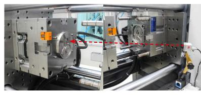
Positioning the infrared camera in the tool installing area
